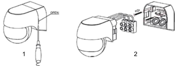
Loosen the screw in the back and unload the bottom (refer to 1).
